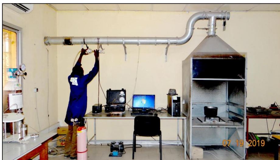
Figure 2: LEMS hood, ducts and gravimetric assembly
