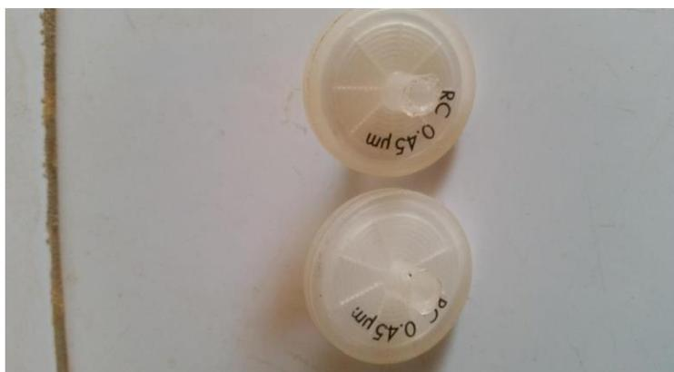
**Figure II:** Photo of 0.45µm microfilter
