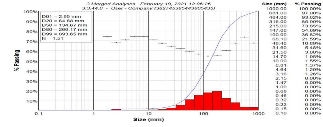
Figure 5: Sieve size curve for shot 1 (emulsion) (blast SMD Iern)
