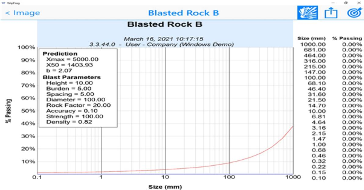
Figure 2: Particle size distribution curve
