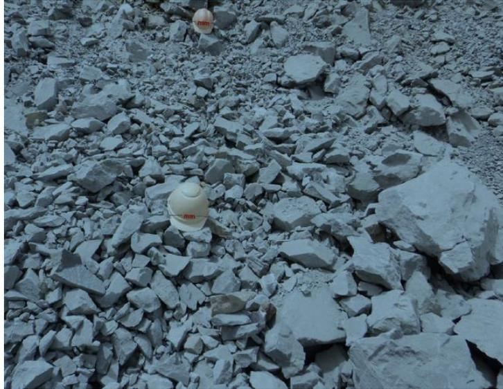
**Figure 4: Illustrative photo of the presence of large blocks (blast SMD lero)**
