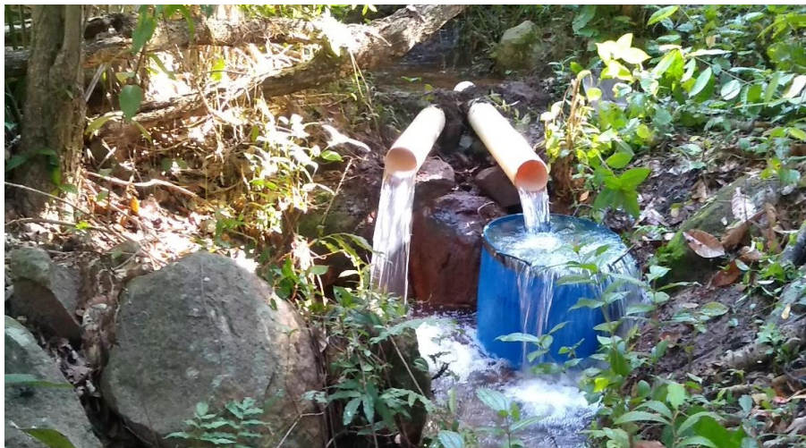
Figure 2 – Flow measurement performed by the volumetric method at FCR005
