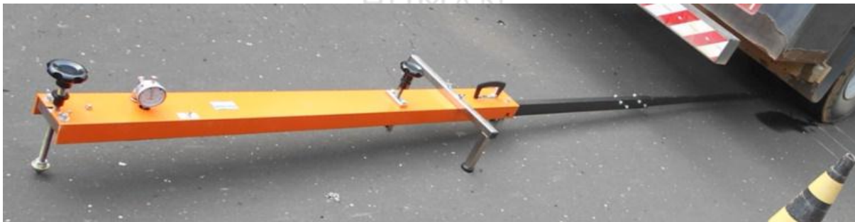
Figure No. 9: Benkelman beam.
