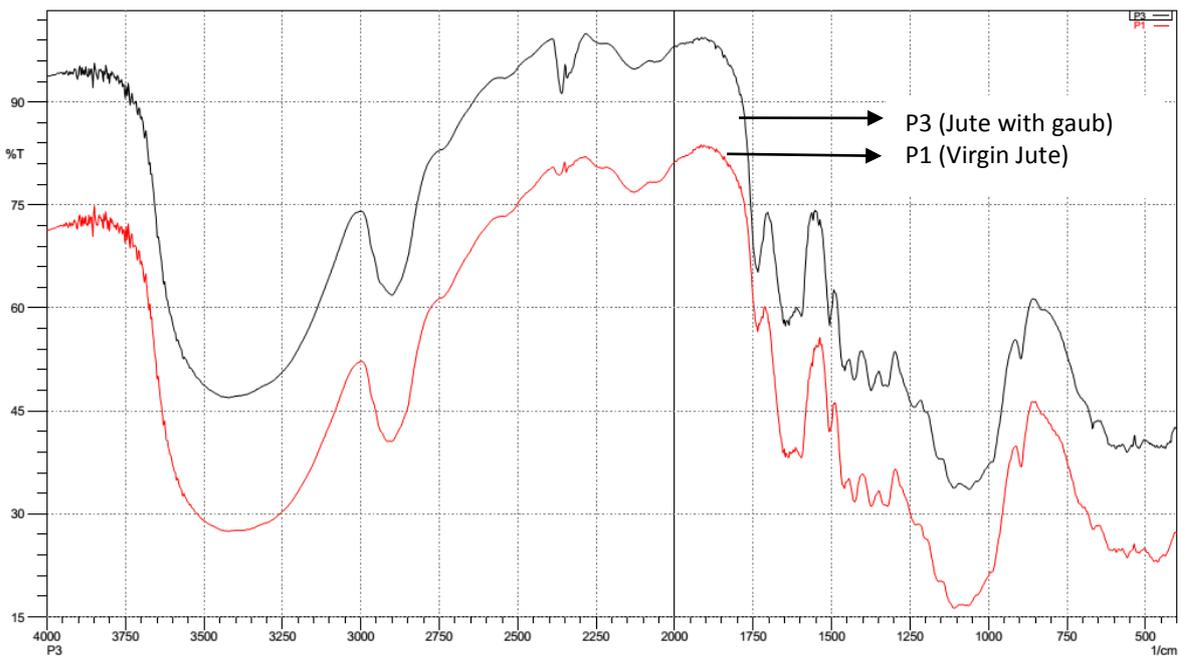
Figure No. 2: P1\_P3: Comparative study of FTIR the virgin jute fiber and treated with gaub as a coupling agent
