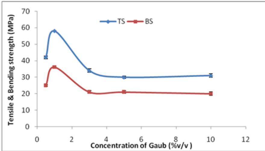
Figure No. 5: The tensile strength (TS) and Bending strength (BS) with the concentration of Gaub
