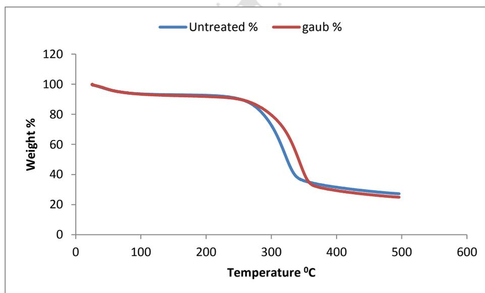
**Figure No. 3: The weight loss by temperature (TGA)**
