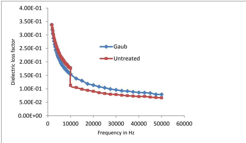
**Figure No. 9: Dielectric loss factor of the composite sample**
