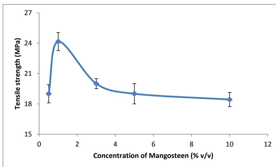
**Figure No. 4: The tensile strength of the treated jute with the concentration of gaub**
