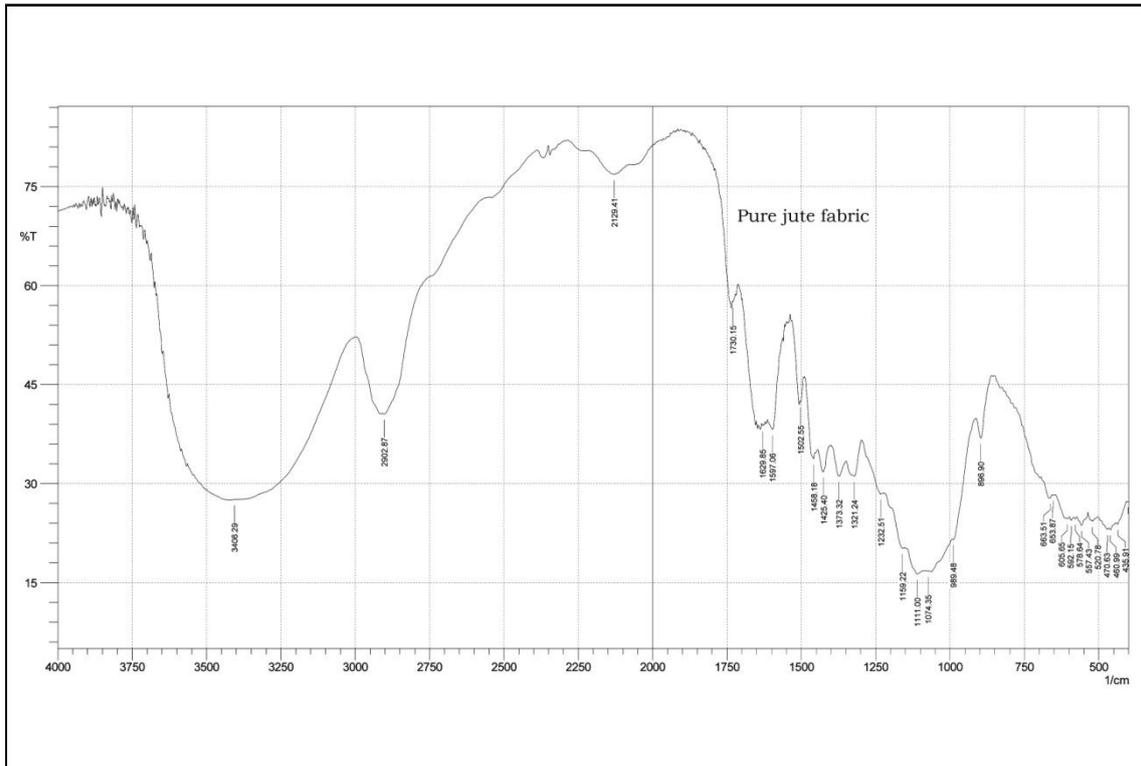
Figure No. 1: The FTIR study of pure Jute fiber
