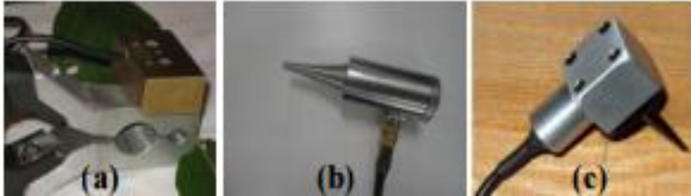
Figure No. 1: Transducers: (a) 30 kHz, (b) 54 kHz (exponential) e (c) 150 kHz
