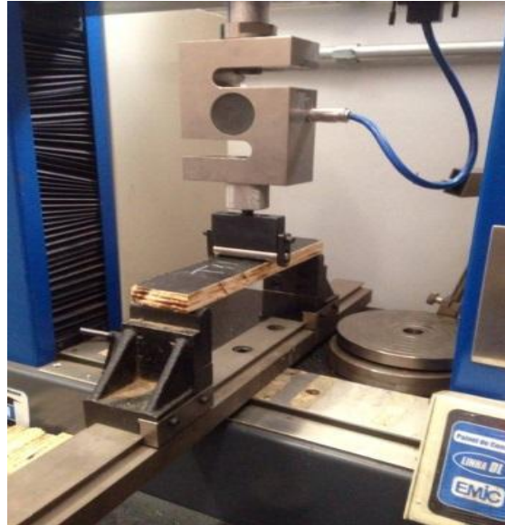
Figure No. 3: Test of static flexion in three points.
