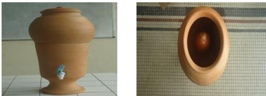
Figure No. 1: Water filtration device
