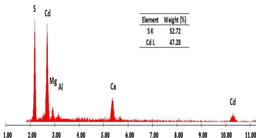
**Figure No. 3: EDX of a typical CdS:K film on glass prepared at. 1 % K**
