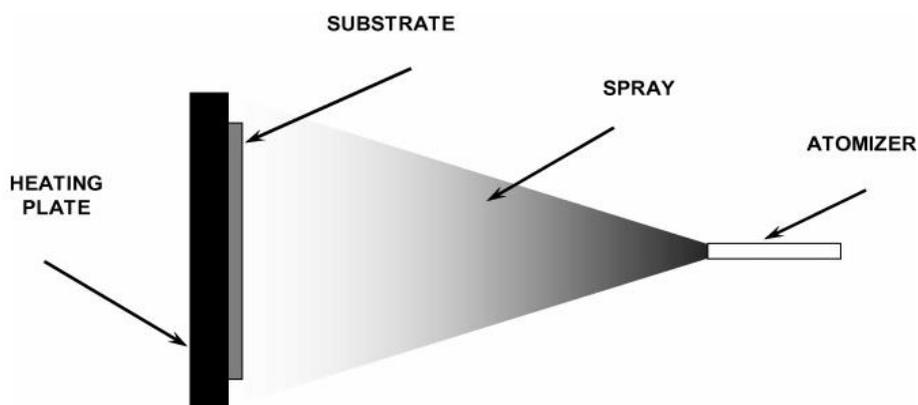
**Figure No. 1: Schematic diagram of spray pyrolysis method**
