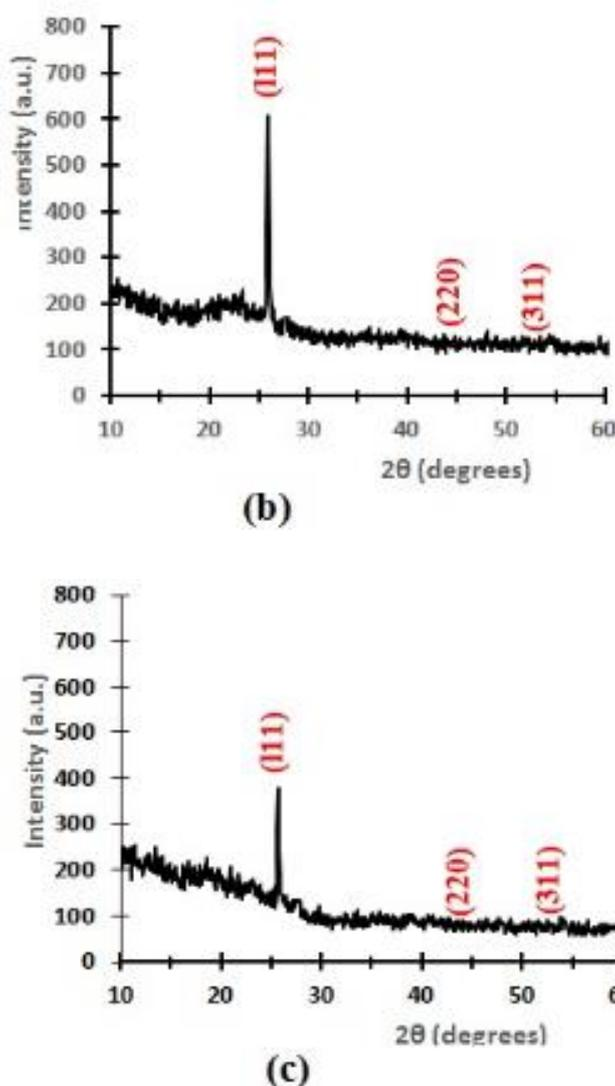
**Figure No. 4: XRD patterns of films deposited at different potassium chloride content (a) 1 at.%, (b) 2 at.% and (c) 3 at.%**
