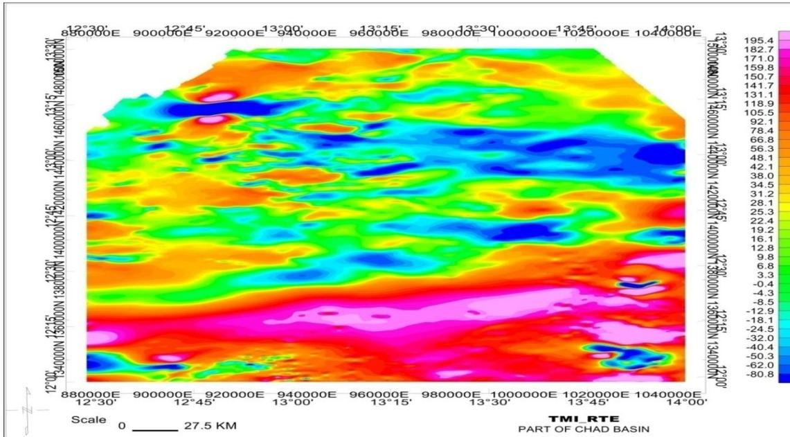
Figure no. 4 Total Magnetic Intensity (TMI) Map of the Study Area Reduced to Equator.
