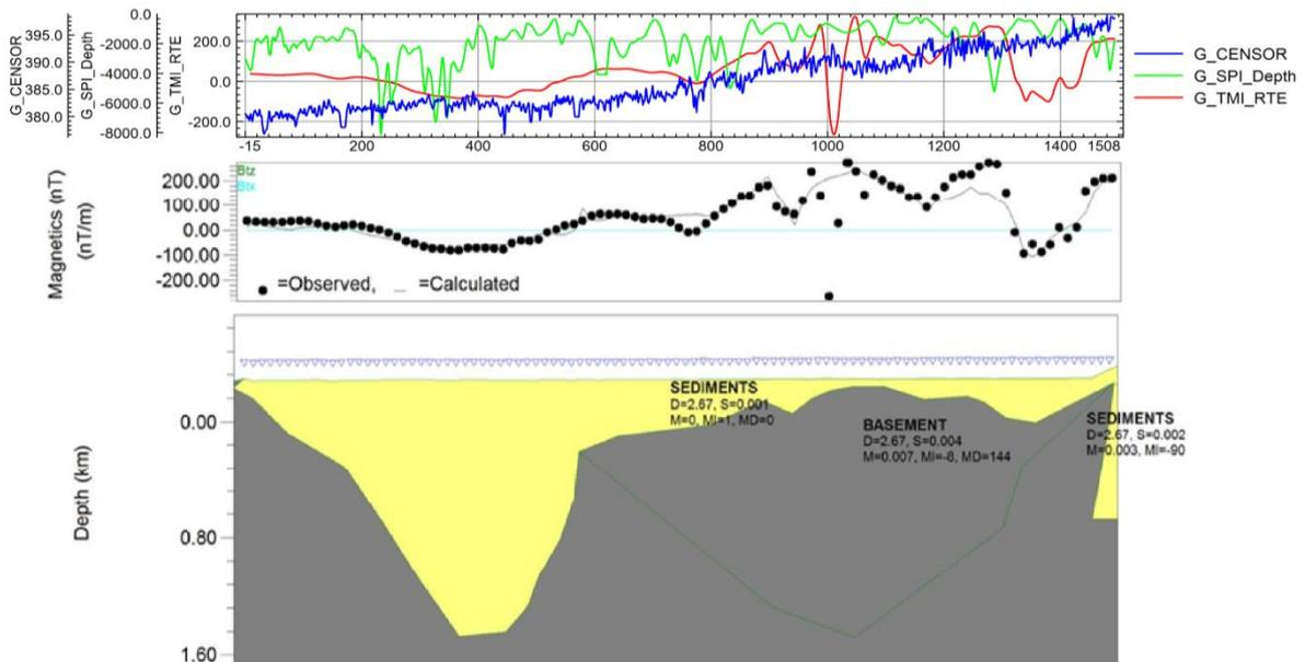
Figure no. 9: Profile and Model Map for profile 2.
