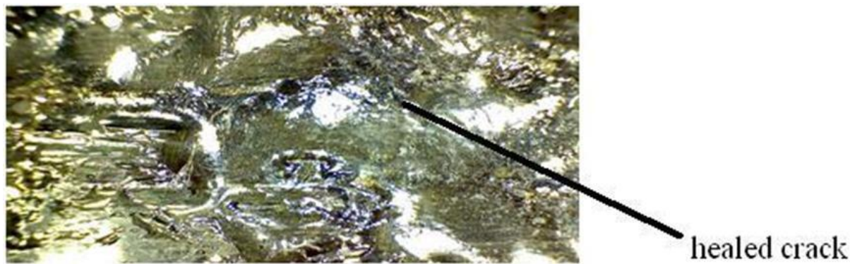
Figure 21: Optical microscope pictures of crack and crack healed sample
