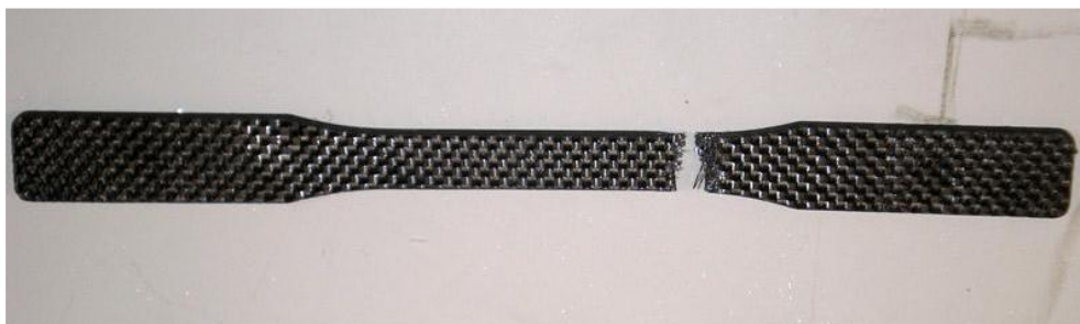
Figure 7: Sample of Self-Healing composite after tensile strength
