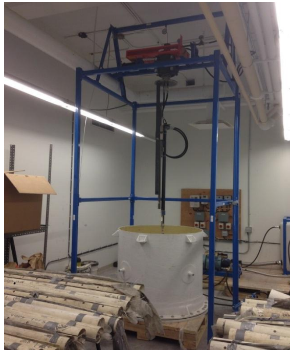
Figure 3: Laboratory jet grouting setup at the UofA
