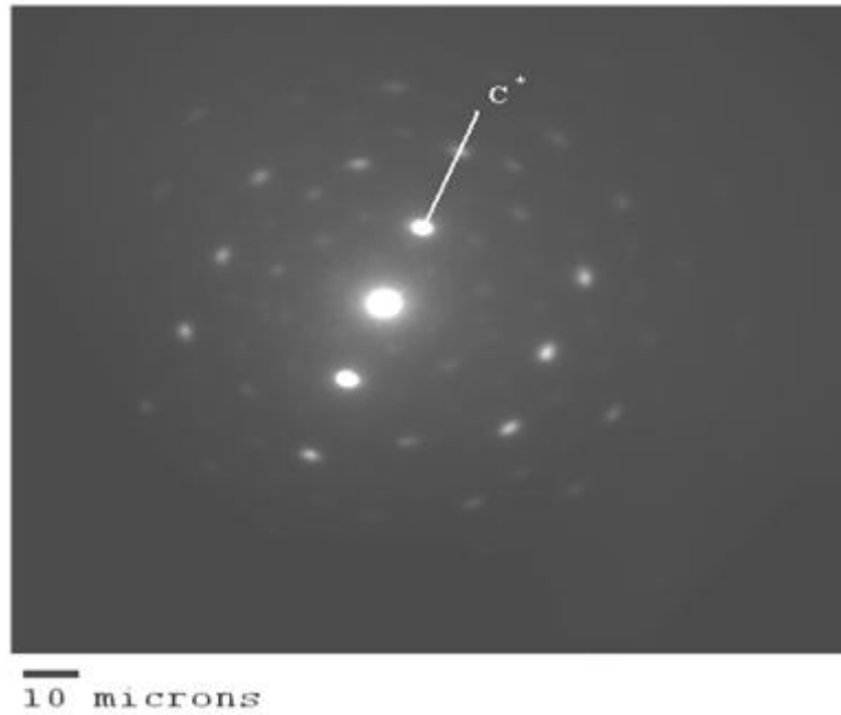
Fig. 11. The selected-area electron diffraction (SAED) of Sohail island biotite showing streaking parallel to c^* in rows caused by the random spacing.
