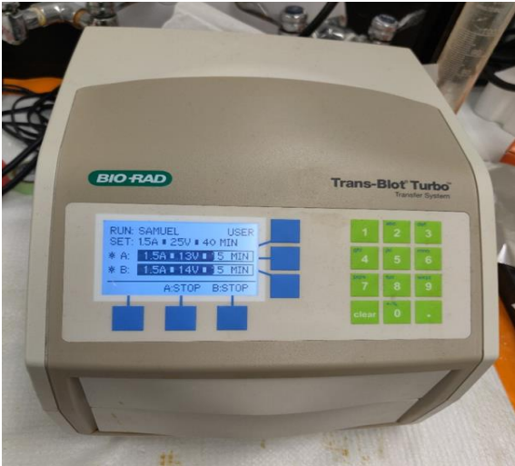
Figure No. 3a: Semi-dry transfer with Trans- Blot Figure No. 3b: Wet transfer Turbo Transfer System
